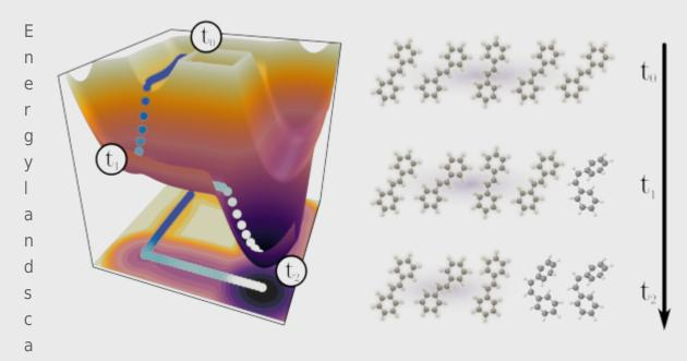
pe that governs the chemical reaction of two molecules after the system absorbs one single photon. At the first reaction step t0 the system consists of five molecules strongly interacting with the electromagnetic vacuum. At the second reaction step t1 the system has evolved and one molecule has isomerized. In the strong coupling regime this process continues with more steps in which one molecule isomerizes after another.
