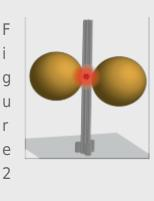
Using this highly confined excitation field we were able to perform single molecule measurements in solution at concentrations as high as  $25\mu M$  in the biologically relevant range. Additionally, we report on a controlled increment of the radiative rate of organic dyes in the vicinity of gold nanoparticles with the consequent increment in the number of total emitted photons [6,7].
